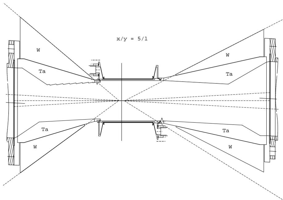
Be: liquid-cooled, Cone: water-cooled.
