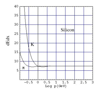
dE in 5 lyrs of 0.3mm-thick Si = 0.6 MeV ( $\sim$  1.5 m of gas) : a Si layer is **'thick'**.
