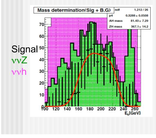
Assuming contributions from all B.G are measured, only signal (points with error bar) is fitted.
