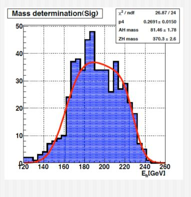
input :  $m_{AH} = 81.9 \text{ GeV},$   $m_{ZH} = 369 \text{ GeV}$ fit results :  $m_{AH} = 81.5 \pm 1.8 \text{ GeV},$   $m_{ZH} = 370 \pm 2.6 \text{ GeV}$ -0.2 $\sigma$  and 0.4 $\sigma$  respectively.
