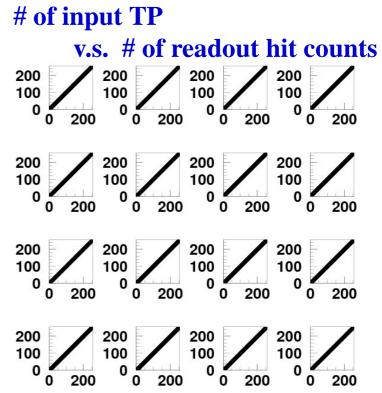
The readout ASIC was confirmed to work correctly as designed.
