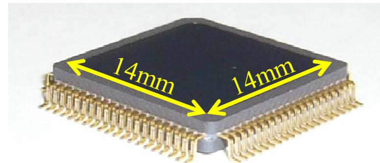
→ Performance of the prototype ASIC was tested.
