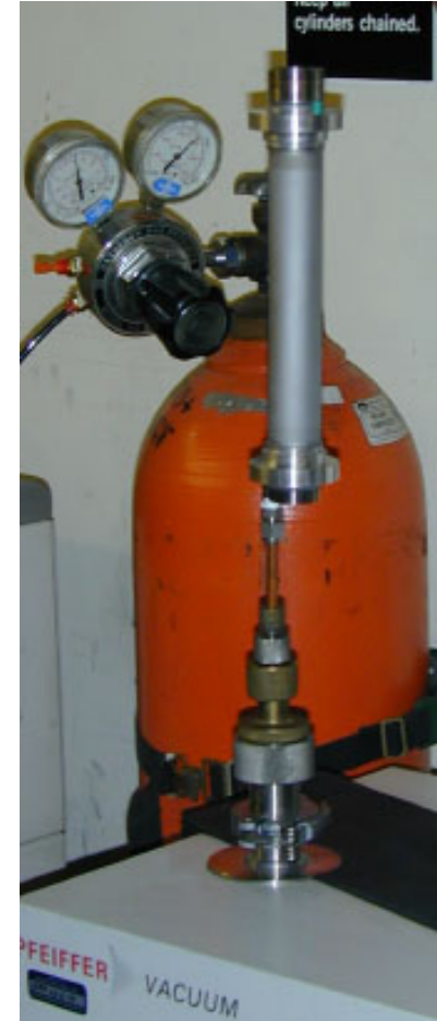
He leak test
