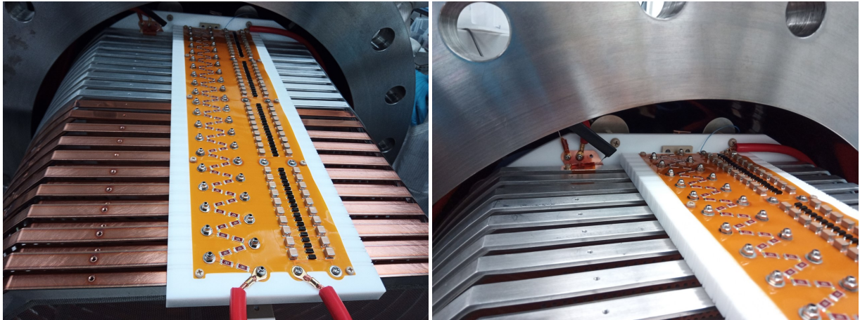
Fig. 3.7 CW and resistor chain are mounted on a PTFE jig and installed on the field cage. The field cage and anode electrode are connected via a resistor FPD4D200MOHMF (black plate seen against the white PTFE at the end of the field cage).
