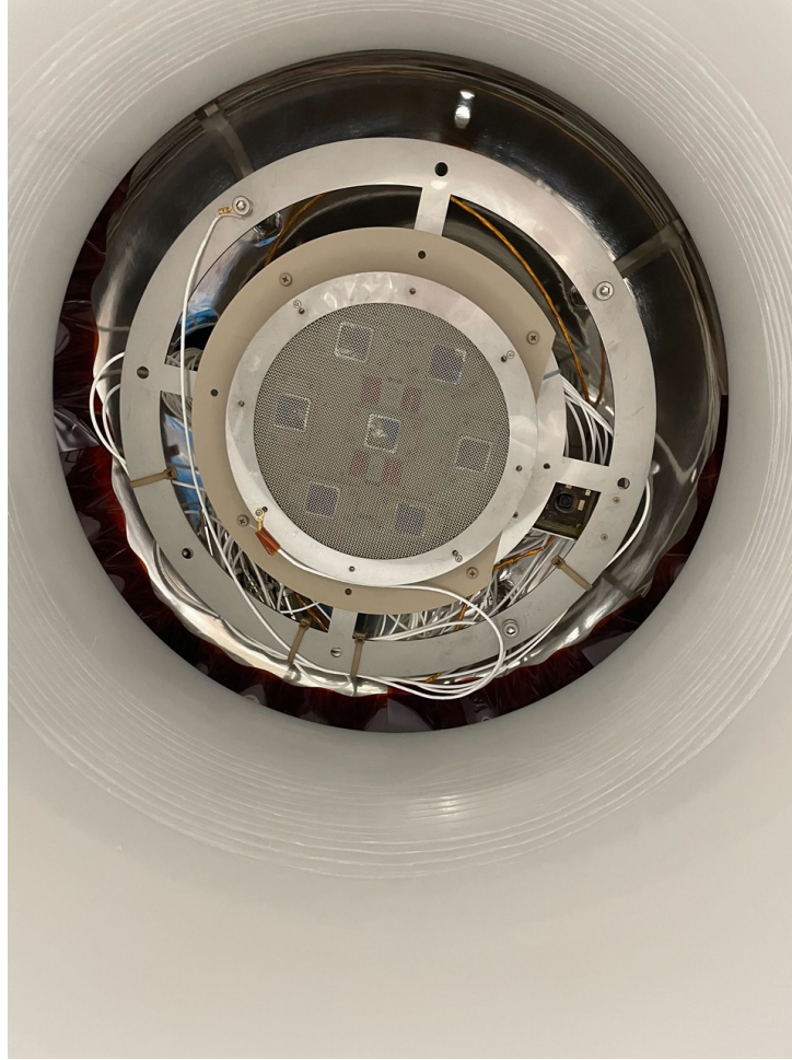
Fig. 3.12 Grooves carved into the HDPE tube as a countermeasure against the discharge. In the background, the PMTs and the guard mesh can be seen.
