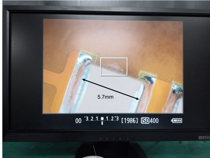
Fig. 3.6 Example of air bubbles remaining in gaps between circuit elements.
