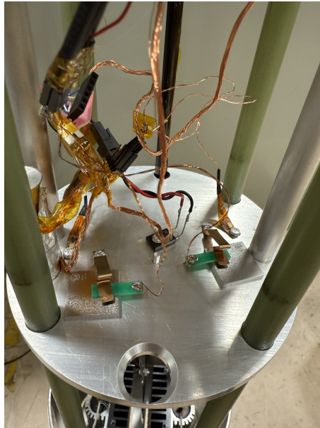
Figure 8.8: The sample stage inside the cryostat.
