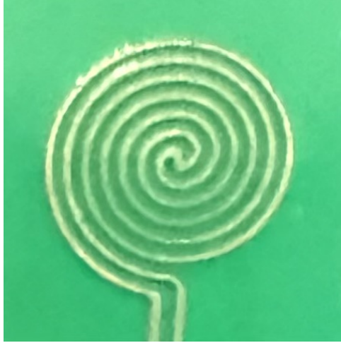
Figure 1.7: The picture of spiral coil used in this thesis. The design of the spiral coil is by Yoshihisa Iwashita(Osaka University).
