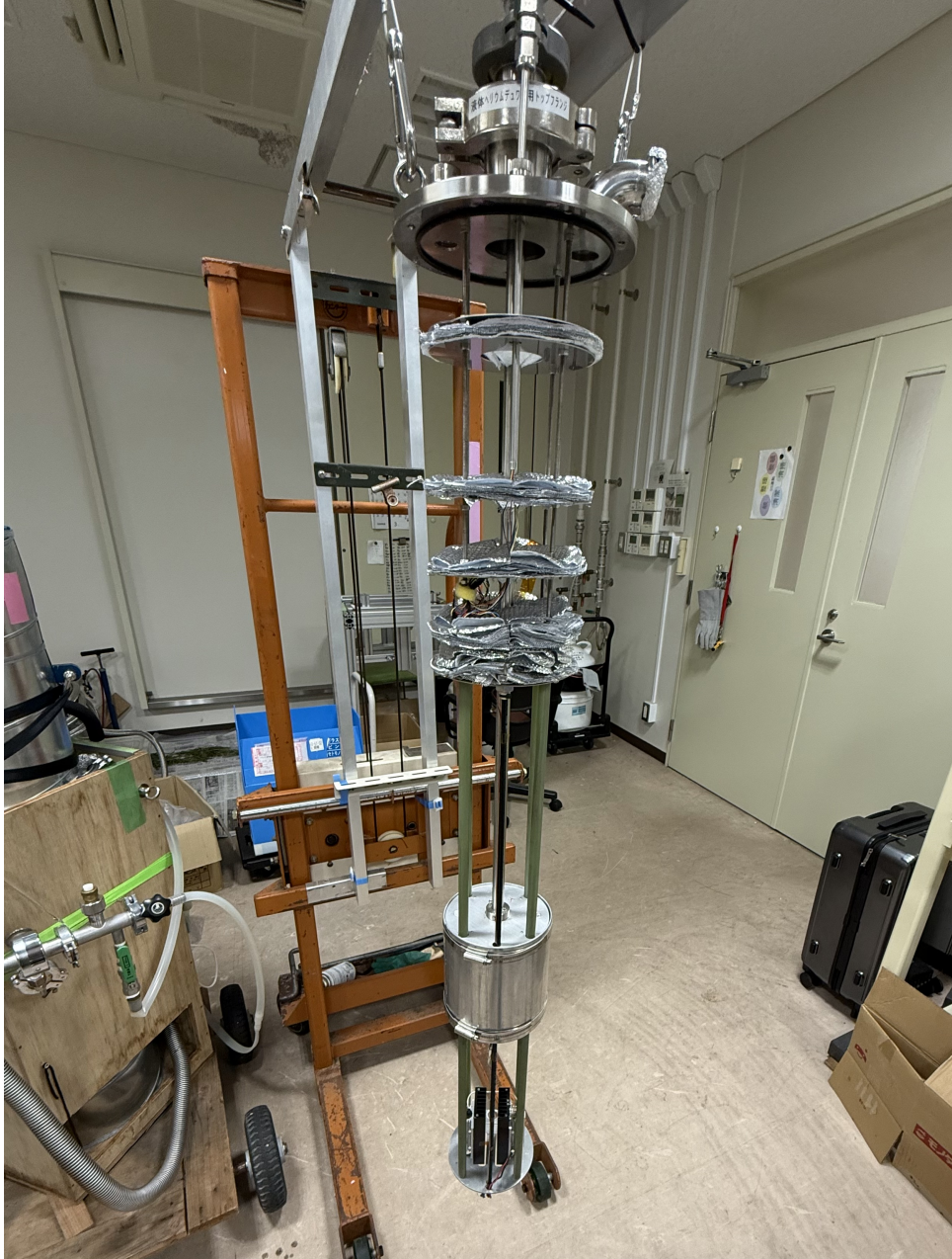
Figure 8.7: The whole inner structure including the baffles for thermal insulation.
