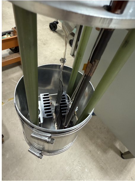
Figure 8.9: Heater and thermal tab connected to the sample stage.
